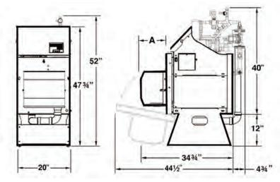
Recommended service clearance: 20" from front door face, 5" left side and 12" right side. Clearance to combustibles: 4" from the rear cover; 10" above top cover; 0" from polypropylene pipe; 0" for all the other dimensions.
